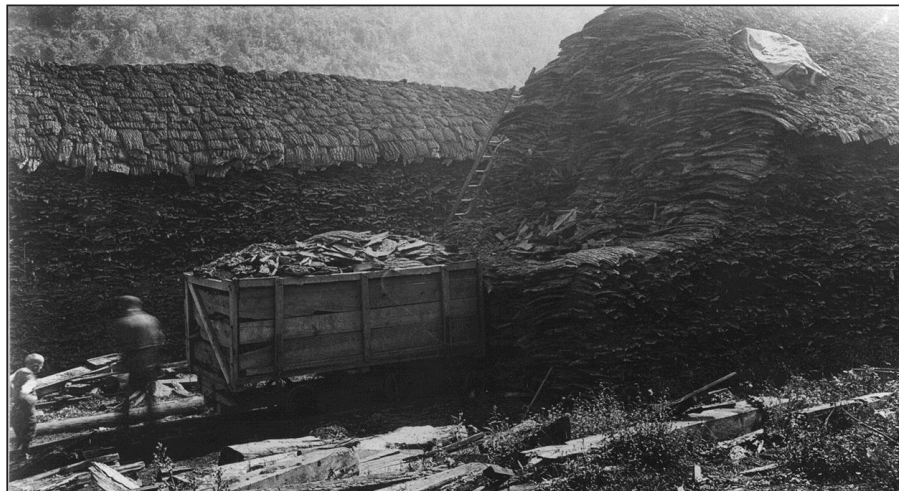
Photo courtesy PA Department of Conservation and Natural Resources Surrounded by piles of Hemlock tanbark, workers fill a railcar with the valuable commodity, harvested for its tannin, which was used in tanning leather. (Photo taken in Leetonia, Tioga County, PA, circa 1900)
